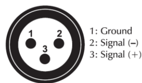
DMX-input XLR mounting-plug:
