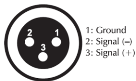
DMX-output XLR mounting-socket:
